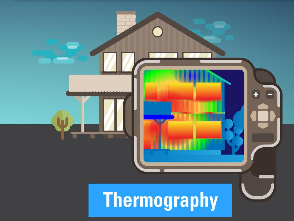
Thermography measures the energy or heat of an object by using an infrared camera. All objects including electrical equipment give off infrared energy. The higher an object's temperature, the more infrared energy it gives off. Excessive heat differentials within electrical components indicate problems within the equipment.
